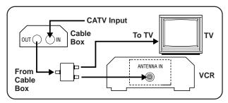
With this connection you can view/record any cable channel <u>including scrambled channels to</u> which you have subscribed.
